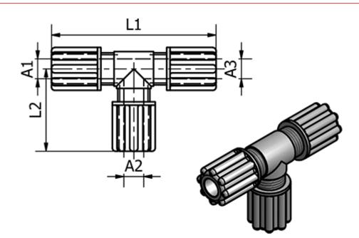
Ext. Hose Diameter A1 = 9/12Ext. Hose Diameter A2 = 9/12Ext. Hose Diameter A3 = 9/12L1 = 74 L2 = 37
